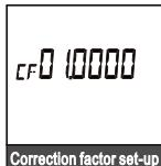
Correction factor set-up : A coefficient can correct deviation
