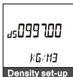
When calculating fluid weight need to set-up liquid density
